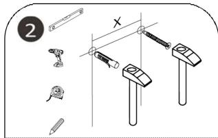
Make marks on the wall with a pencil and ensure they are on the same level before drilling guide holes. Insert the expanding rubber plugs into the holes first, and then drive in the long screws.
