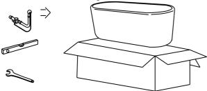
Adjust the foot screws to land all its feet, meanwhile adjust it to a level which can drain water smoothly.
